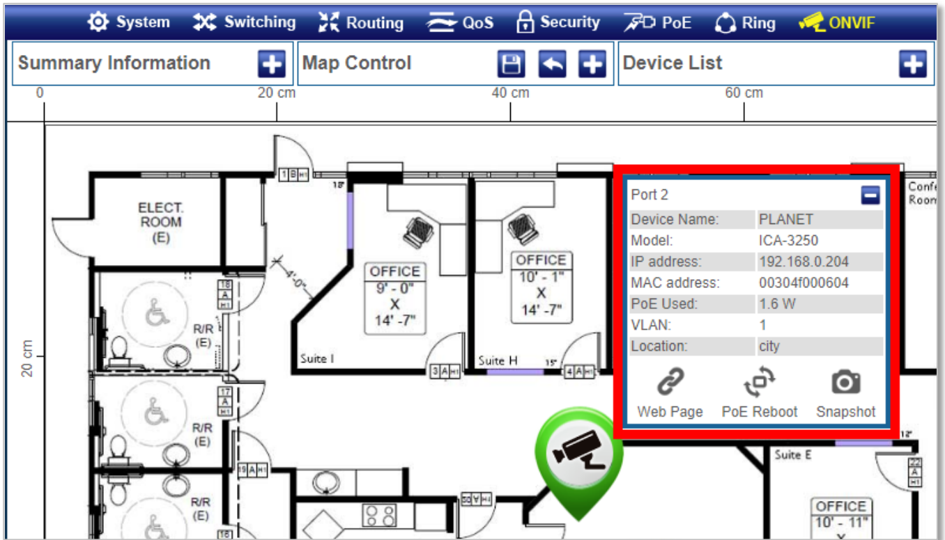
Figure 4-9-5-3: Floor Map Page Screenshot – Display device information of selected ONVIF IP camera
